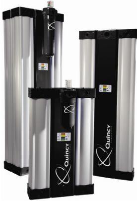
Quincy Compressor's **Q Mod heatless desiccant dryers** deliver clean, dry air to the point of use by filtering liquids and adsorbing water vapor from a compressed air stream. Air is initially directed through a 0.01 PPM polishing pre-filter, removing untreated compressed air full of liquids, aerosols and mists. The high-tech dryers offer:
