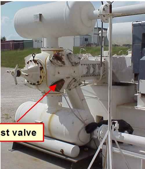
*Figure 14: Ariel Reciprocating Compressor Used in Measuring Valve Motion*
