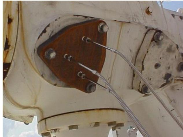
*Figure 15: Ariel Reciprocating Compressor with Optical Position Probes Mounted on Valve*
