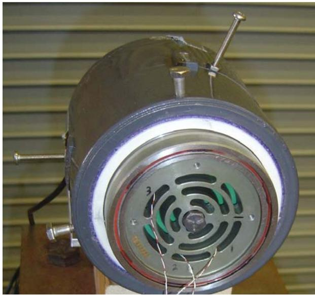
Figure 5: Instrumented Valve Fixture
