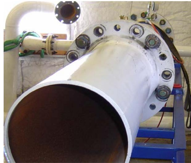
Figure 4: Burst-Membrane Shock-Tube
