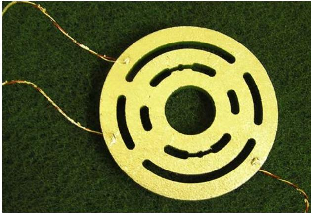
*Figure 6: Valve Plate with Reflective Coating and Mounted Strain Gauges*
