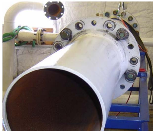
Figure 4: Burst-Membrane Shock-Tube
