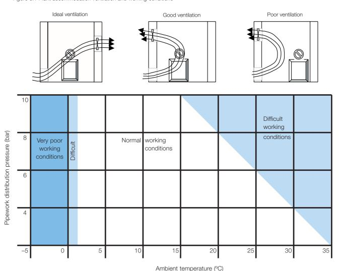
Figure 3.1 Plant accommodation ventilation and working conditions
