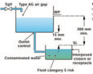
**Type AUK1 air gap with interposed cistern**. This provides back-flow protection to fluid category five. The air gap in the cistern must meet the requirements for a type AG air gap (British Standard BS6281: Part 2).
