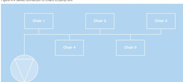
Figure 4.4 Series connection of chairs to pump unit
