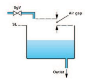
**Type AA air gap, with unrestricted discharge**. This provides back-flow protection to fluid category five. The discharge point is located above the spillover level (SL) of the receptacle. The minimum distance between the discharge and the spillover level must meet the requirement for a type AA air gap.
