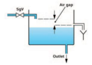
**Type AF air gap with circular overflow**. This provides backflow protection to fluid category 4. The dimension of the air gap between the discharge point and the 'critical water level' (water level two seconds after closing the inlet) must meet the minimum requirements for the standard.
