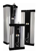
Quincy Compressor's **Q Mod heatless desiccant dryers** deliver clean, dry air to the point of use by filtering liquids and adsorbing water vapor from a compressed air stream. Air is initially directed through a 0.01 PPM polishing pre-filter, removing untreated compressed air full of liquids, aerosols and mists. The high-tech dryers offer:
